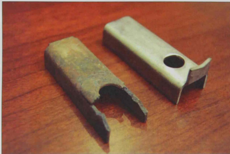
Figure 2: Severely corroded stainless steel 316L clip next to a new one
