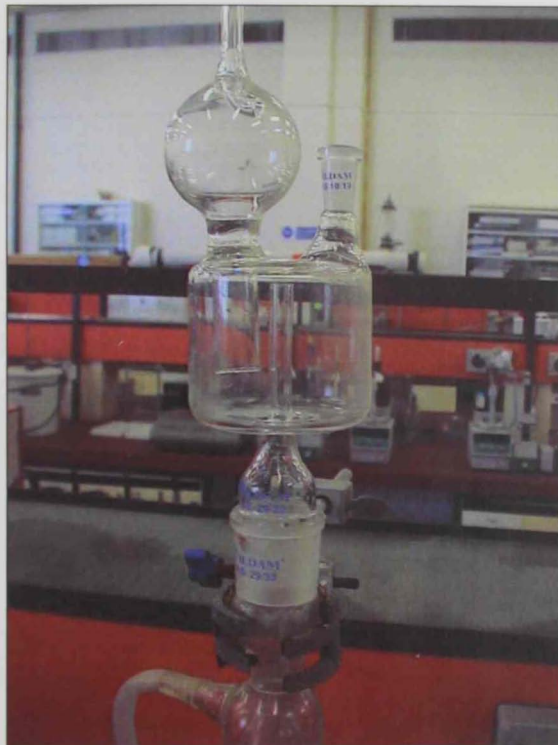
Figure 24: Assembled apparatus with a close up of water condenser and trap
